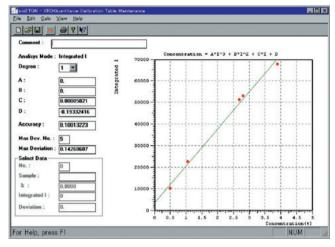
Calibration Curve Screen for Integrated Intensity
