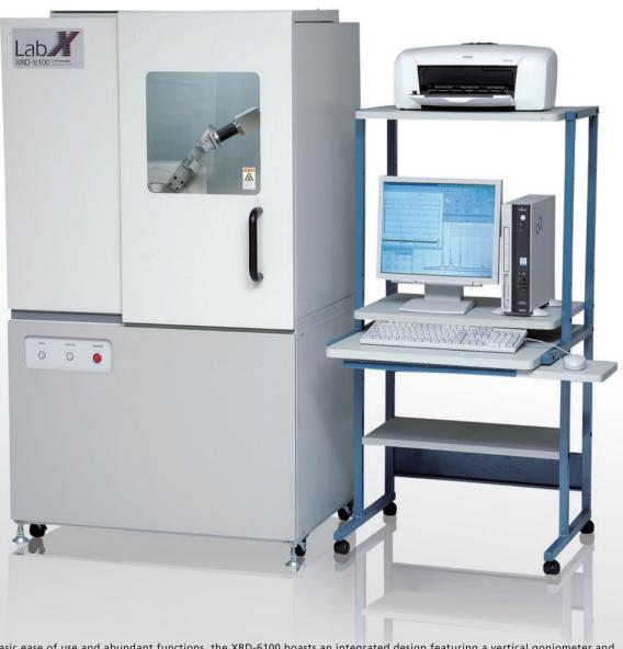
In addition to its basic ease of use and abundant functions, the XRD-6100 boasts an integrated design featuring a vertical goniometer and data processing software supporting the Windows 7 user interface.
