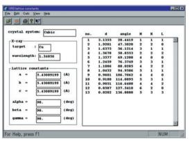
Precise Lattice Constant Determination Calculation Result Screen
